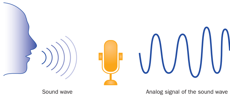
FIGURE 1.3 A sound wave and an electronic analog signal that represents the wave
