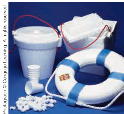
Blowing agents—such as hydrazine, which forms nitrogen gas on decomposition—are used to produce porous plastics like these polystyrene products.
