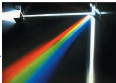
Spectrum obtained by shining a beam of light at an angle to a diffraction grating.
