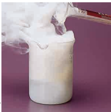
Liquid titanium(IV) chloride being added to water, forming a cloud of solid titanium oxide and hydrochloric acid.
