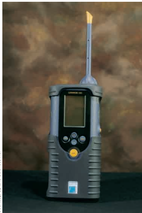
A Cyranose sensor (an “electronic nose”).
