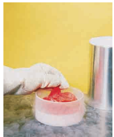
The balloon collapses as the molecules inside slow down because of the decreased temperature. Slower molecules produce a lower pressure.
