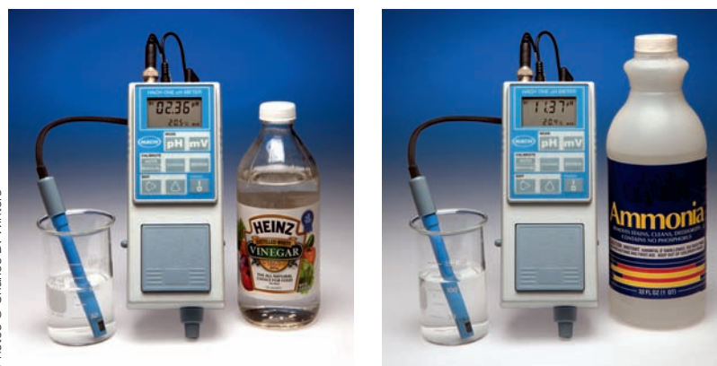
Figure 7.4 (a) Measuring the pH of vinegar. (b) Measuring the pH of aqueous ammonia.
