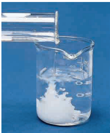
The precipitation of lead(II) sulfate by mixing solutions of lead(II) nitrate and sodium sulfate.
