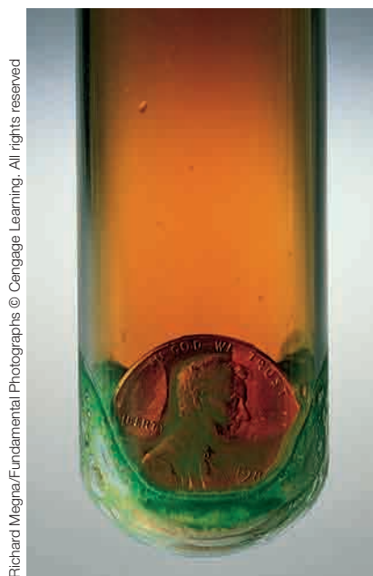
A copper penny reacts with nitric acid to produce \text{NO} gas, which is immediately oxidized in air to give reddish brown \text{NO}_2 .
