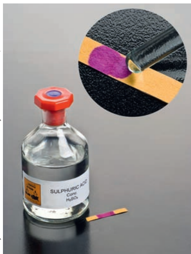
A bottle of sulfuric acid. A drop of sulfuric acid turns Universal indicator paper bright red, showing it is very acidic.
