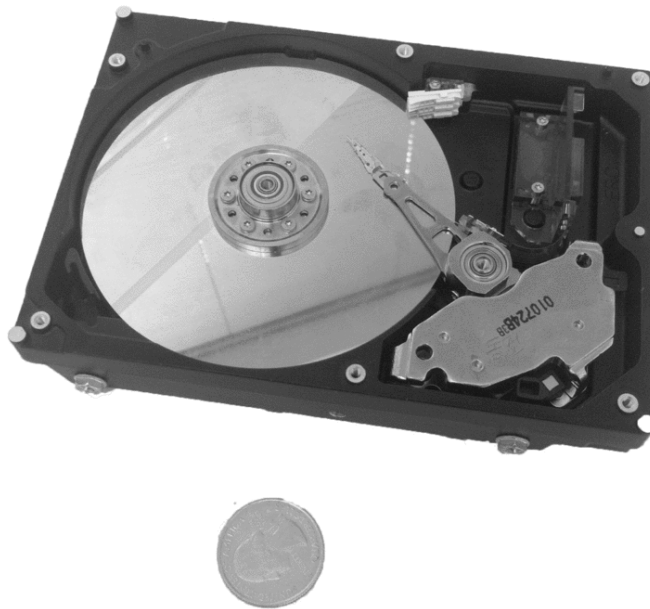
Figure 12.1: A partially-disassembled magnetic disk drive.
